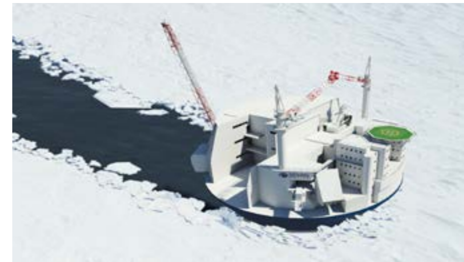
Cylindrical hull concept – Arctic Ice hull (Source: Sevan Marine)
