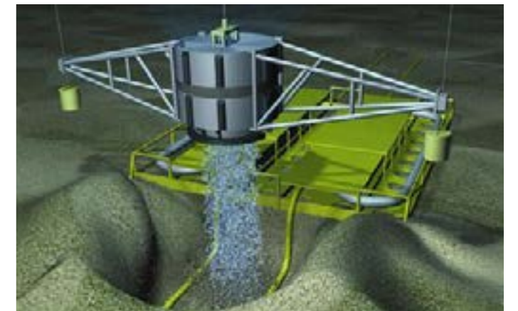
HydroDigger excavation system (Source: Scan Tech)
