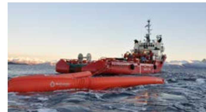
Arctic Oil Spill Boom (Source: Norlense)
