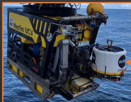
Sensor frame with three relative gravimeters and three pressure sensors
